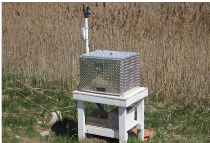
Hydrogen Sulfide monitor located downwind of landfill
