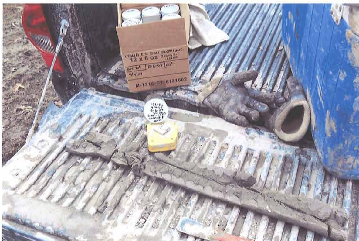
Photograph 2.2-3 Typical Lower Till Sample Obtained with Split-Spoon Sampler
