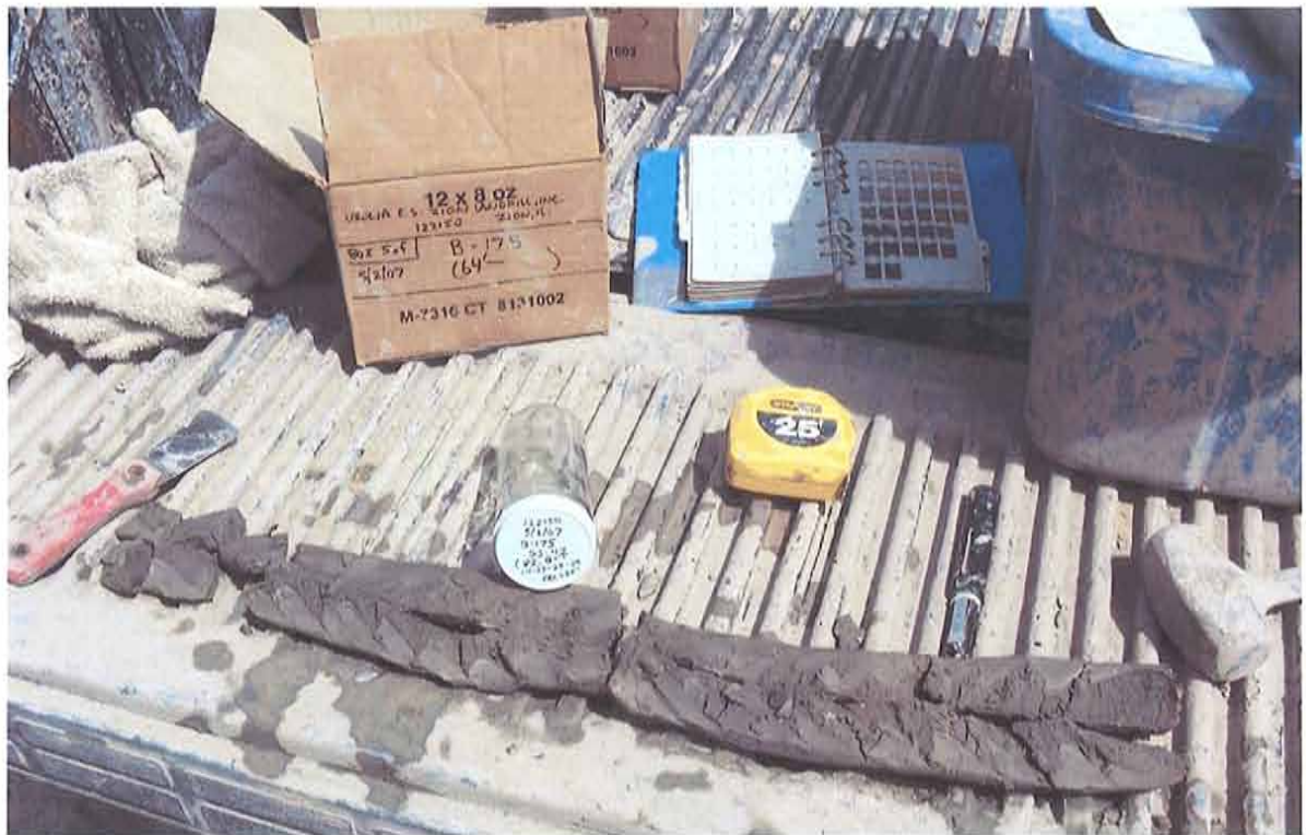
Photograph 2.2-2 Typical Wadsworth Formation Sample Obtained with Split-Spoon Sampler
